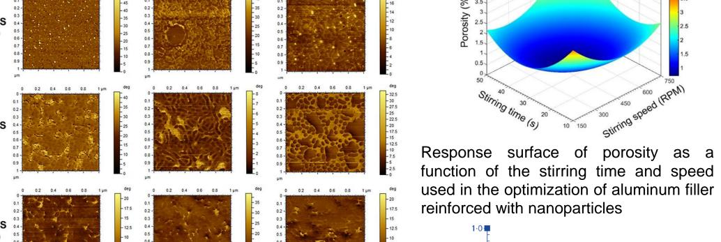
AFM phase images for the sulfonated and Poly (styrene isobutylene - styrene) nano-composites membranes with maximum nanofiller loadings.
