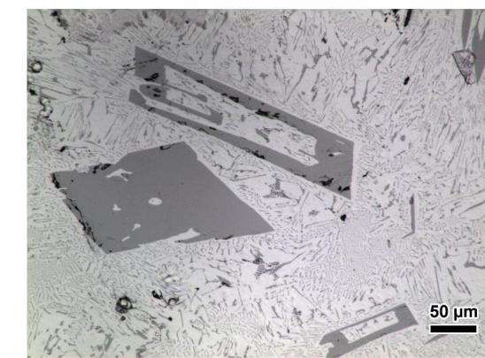
Optical image of the microstructure of the external surface of a centrifugally experimental AI - 14wt.% Ce sample. The 500 RPM rotational speed allowed segregating the largest intermetallic particles of this
