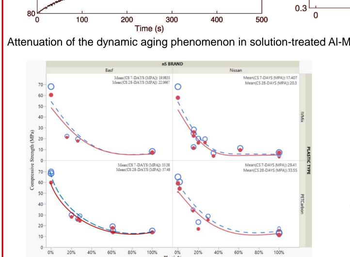
Compressive strength of nanomodified concrete proposed as structural material containing recycled plastic and different types of nanosilica.
