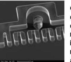
GOAL: develop scanning probe microscopy (SPM) for quantitative measurements of mechanical and chemical surface properties at the nanoscale. Our method is based on measurement of time-resolved interaction forces between the atomic force microscope (AFM) tip and the sample surface by using a micro-machined cantilever with an integrated high-
