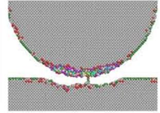
GOAL: enabling the simulation and understanding of the interaction of an AFM tip with samples of different stiffness. We are exploring practical ways of utilizing time-resolved force information to expand the applicability of AFM as a measuring tool and enhance its reliability. The current focus is in exploring the reliability of local mechanical properties of the sample through continuum mechanics and atomistic models.
