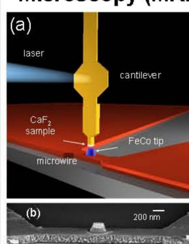
develop a microscope that can ultrasensitive force detection of nuclear magnetic resonance force microscope include the development of sharp magnetic tips that produce field gradients over 14 gauss per nanometer and a lithographically fabricated copper "microwire" that allows a 40 gauss rf field to be generated with less than 500 microwatts of heating. ("Nuclear magnetic resonance imaging with 90-nm resolution," Mamin, et al., Nat Nano 2:301
