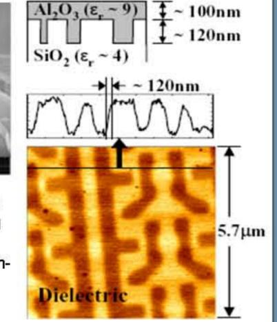
FIGURES: SEM image of the probe end, showing the excitation electrode and the Pttip deposited by FIB. Flat sample with sub-surface dielectric contrast. The NSMM image shows clear contrast in the dielectric channel with ~120nm spatial resolution. (Shen, Kelly, Lai)
