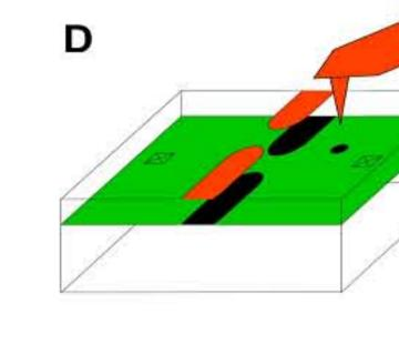
Figures: D: SGM schematic showing metallic gates and tip, orange, creating depletion regions, black, in the 2DEG, green, buried below the surface of the sample. B: Electron flow originates from the QPC formed between two depletion regions (black). Red arrows denote branch points where one branch splits into two. (Goldhaber-Gordon, Jura, Sciambi)
