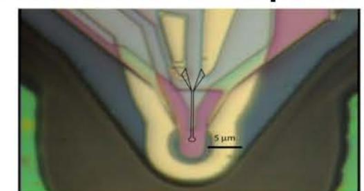
GOAL: develop an ultra-sensitive, high resolution Superconducting QUantum Interference Device (SQUID) Microscope to measure magnetic flux. Recent efforts have focused on defining a lithographic touch down point on the tip (lower purple tab). This point will bring the sensor within 100 nanometers of the sample. (Moler, Koshnick)
