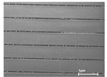
Fig 2B. 50 nm PSL nanoparticles in 50 nm trenches
