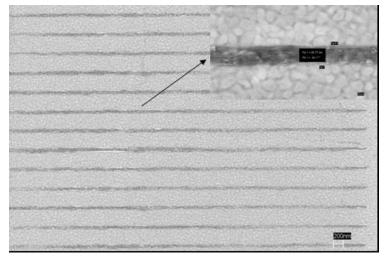
Fig 3. Assembly of SWNTs into sub 100 nm trenches
