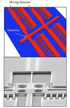
Fig. 4. MEMs Nanowire Tensile Tester for conducting nanoscale tensile test of suspended nanowire using electrostatic combdrive actuator.
