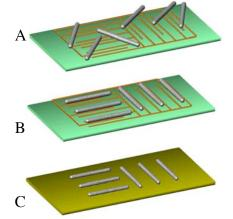
Fig. 1 Nanotubes deposited on template (A), assembled on a nanotemplate (B), and then transferred to second substrates (C).
