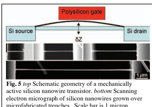
**Fig. 5** top Schematic geometry of a mechanically active silicon nanowire transistor. bottom Scanning electron micrograph of silicon nanowires grown over microfabricated trenches. Scale bar is 1 micron.
