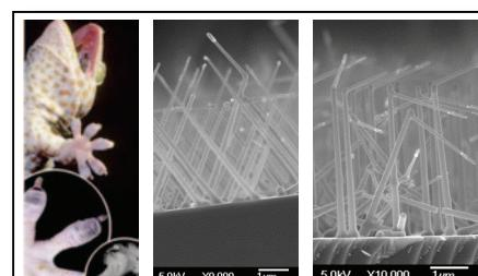
**Fig. 4** *left:* Gecko feet shown at progressively greater magnification, culminating in an image of the nanoscopic setae (lowermost inset). *middle:* Kinked silicon nanowires grown on (111) oriented substrate. *right:* Kinked silicon nanowires grown on (110) oriented substrate.
