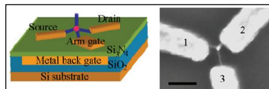
**Fig. 1** Scheme of tetrapod single electron transistor. *left:* the device schematic structure, in which three arms of a tetrapod are contacted with small metal electrodes and the fourth arm points vertically away from the substrate. The fourth arm serves as a mechanical lever acting on the
