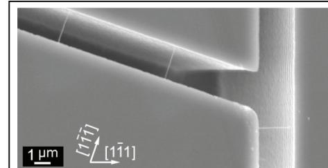
**Fig. 3** Scanning electron micrograph showing rationally-synthesized silicon nanowires bridging microfabricated trenches.
