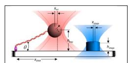
Figure 3. Optical trapping instrument with two detector lasers to subtract out stage noise. One laser (*blue*) tracks the stage noise in three dimensions. The second laser (*red*) tracks the motion of the bead in the trap (*dotted red*).
