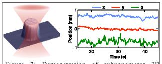
Figure 2: Demonstration of subnanometer 3D stabilization of an optical microscope.
