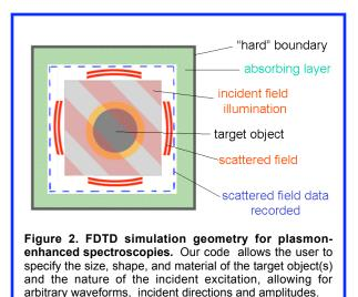
The theoretical analysis and design tools developed in the course of this project will be used to develop a comprehensive understanding of the local electromagnetic environment of plasmonic nanostructures. The principal theoretical approach that will be used is the Finite-Difference Time-Domain (FDTD) discrete method (Fig 2). This method involves the discretization of Maxwell's equation on a spatial grid and the propagation of the local electric and magnetic fields in real time. Our plans are.
