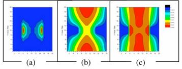
Fig 4: Volume fraction profiles of chain between two electrodes a) adsorbed on a single electrode b) adsorbed on a electrode but not spanning c) spanning the two electrodes.
