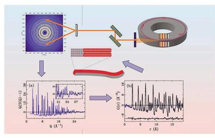
The approach makes use of high-quality x-ray or neutron scattering data from powerful modern national user facilities such as the Advanced Photon Source at Argonne National Lab., combined with advanced computing and novel modeling methods to extract the structural information. The approach is illustrated schematically in the Figure. The scattering data are carefully processed and
