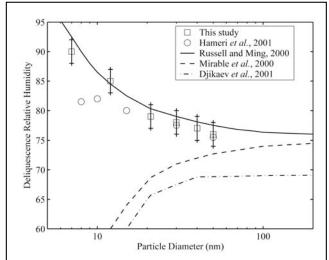
Figure 2. Deliquescence relative humidity of sodium chloride versus particle mobility diameter. Lines: theory. Points: data.
