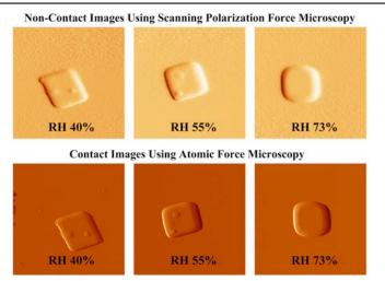
Figure 1. The scanning polarization force microscope (SPFM), a non-contact variant of the atomic force microscope (AFM), is employed to study the hygroscopicity and phase transitions of model atmospheric particles. (Image scale: 3.7 \_m \_ 3.7 \_m)
