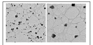
Figure 3. (left) Imaging of NaCl particles at low relative humidity at 283 K. (right) Image of same region after increasing RH above 75% and then returning to low RH. (Image scale: 9.0 \_m \_ 9.0 \_m)
