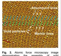
demonstrating the assembly of gold nanoparticles along precision attachment lines on a DNA scaffolding. Marker lines have a similar DNA structure but are designed to remain particle-free. (Blue and green segments indicate line positions. Markers are 64 nanometers apart.) DNA scaffolding is a flat structure formed by the self-assembly of about two-dozen different types of single-stranded
