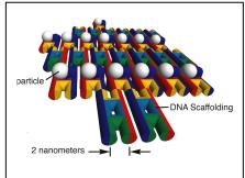
Fig. 1. Schematic diagram illustrating programmed the assembly of nanoparticles along attachment lines on a DNA scaffolding. Colored segments represent DNA strands that selfassemble into a fabric-like repetitive structure. Particles and other nanocomponents precisely attach to the scaffolding along lines by Watson-Crick base pairing.
