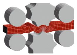
A specific purpose of such simulations is the optimization of designs for tooling such as shown in Figure 2. The simulations therein and as illustrated in Figure 1 are meant to fully optimize the designs to achieve, *inter alia*, maximum uniform shear, but with high levels of hydrostatic compression.
