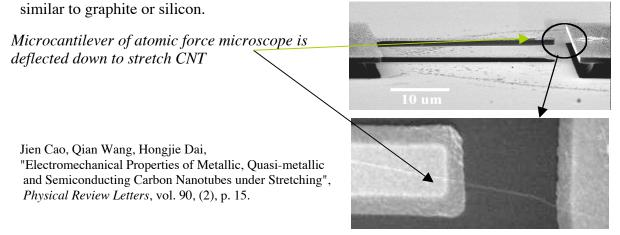
By bending the SWCNT the metallic region is highly confined (to the bend) (left picture, below) offering great possibilities for new sensors (e.g. for bio-chemicals) and other devices such as a very low-noise source of free electrons (right picture) for high speed analog-to-digital conversion (for secure communications).
