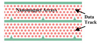
Left: a block copolymer forms an ordered structure in a 260nm wide silica groove. The notch on the side of the groove (red circle) pins the lateral position of the array. Right: a sketch of a magnetic storage medium consisting of nanomagnets arranged in circumferential tracks around a disk. Such a structure could be formed by using the ordered block copolymer as a template.
