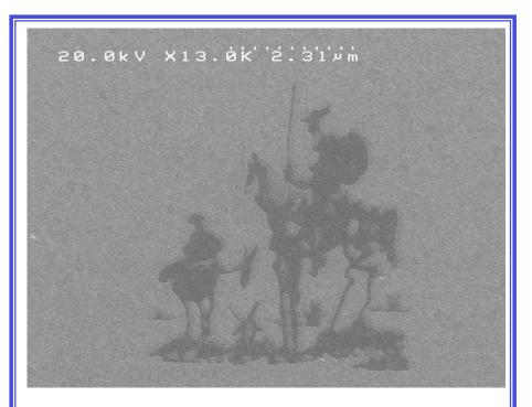
Scanning electron micrograph of Picasso's pen-and-ink sketch of "Don Quixote" in VO<sub>2</sub> (dark color) on an indium-tin-oxide waveguide. The smallest feature size (Don Quixote's spear) is less than 50 nm across.
