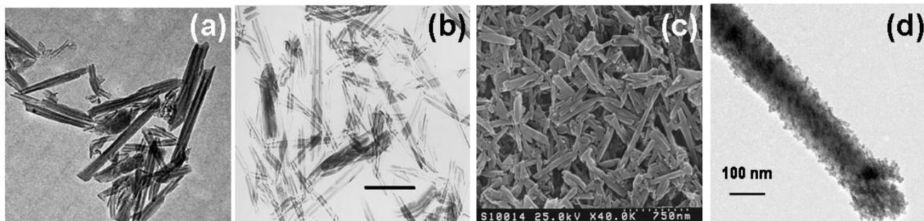
TEM images of halloysite nanotubes dispersed in water, scale-bar 1 μm (a-b), SEM image of layer-by-layer nanocoating with halloysite multilayer (c), and halloysite nanotube coated with polyelectrolyte + 7 nm diameter silica
