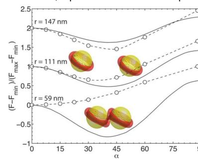
Potential of mean force for association between two nanoparticles (50 nm diameter) suspended in a nematic liquid crystal. \* The approach angle between the Saturn rings and the director is denoted by  $\alpha$ . The lines represent a theoretical approximation by Ruhwandl and Terentjev, and the symbols represent full numerical calculations performed by Thrust 3.
