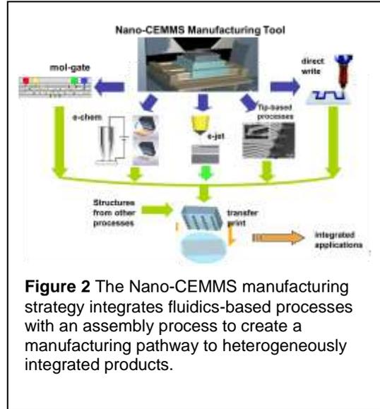
**Figure 2** The Nano-CEMMS manufacturing strategy integrates fluidics-based processes with an assembly process to create a manufacturing pathway to heterogeneously integrated products.
