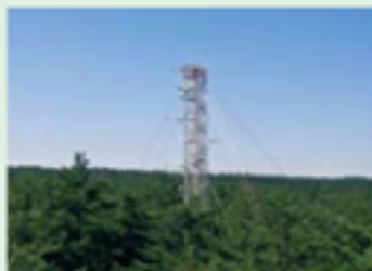
Tower flux observation site measuring CO 2 balances of forest at Mt. Fuji (courtesy of the Forest and Forest Products Research Institute)
