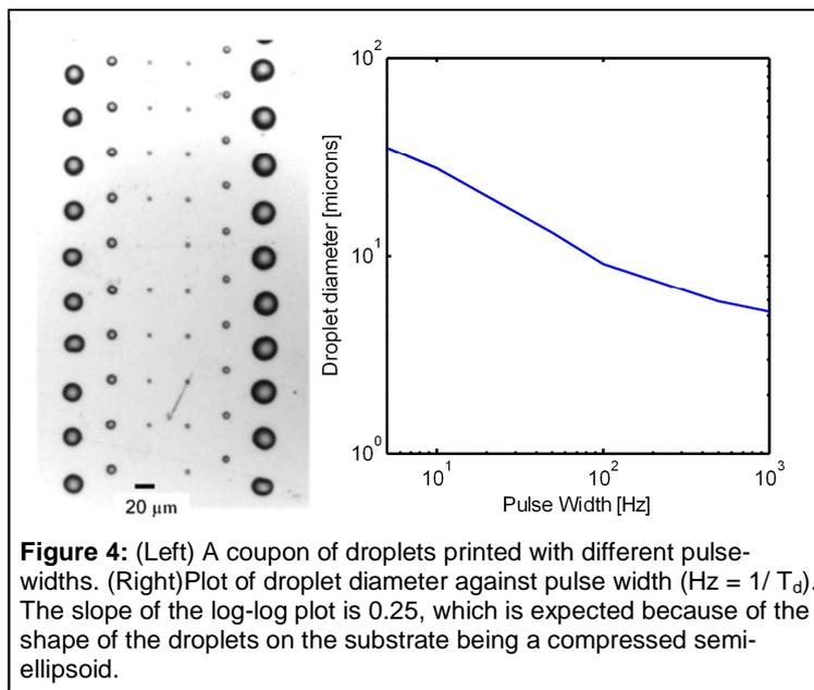
**Figure 4:** (Left) A coupon of droplets printed with different pulse widths. (Right) Plot of droplet diameter against pulse width ( $\text{Hz} = 1/T_d$ ). The slope of the log-log plot is 0.25, which is expected because of the shape of the droplets on the substrate being a compressed semi-ellipsoid.
