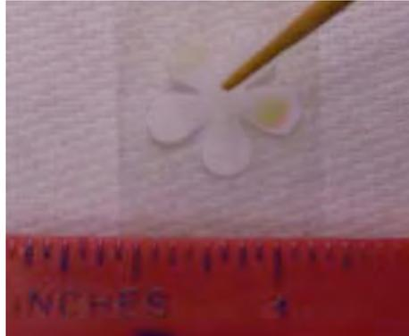
Paper diagnostics prototype for the K-12 classroom made with chromatography paper and a craft punch. Reagents for standard assays for pH and protein are dotted on each “petal” and sample is loaded in the center with a toothpick. Capillary action causes the sample to travel to all petals; a color change indicates pH and protein.
