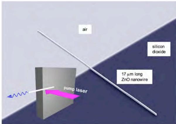
We have measured, for the first time, the output power of a single semiconductor Zinc Oxide nanowire laser emitting in the ultraviolet. The figure shows the experimental configuration: A nanowire, partially suspended in air, is excited uniformly along its entire
