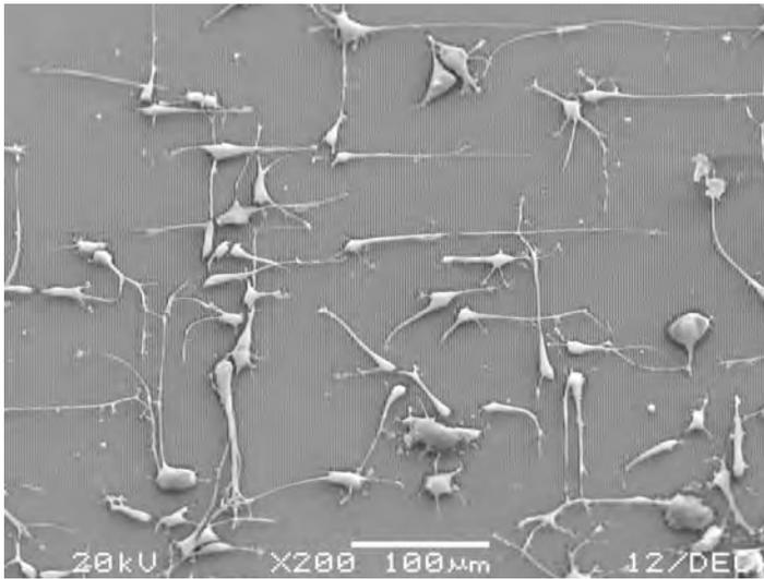
Nanopost arrays with tailored size, spatial distribution, and chemistry were fabricated to control stem cell differentiation. Such nanostructures seem to induce distinct morphological characteristics in stem cells that resemble neuronal architectures. Further studies
