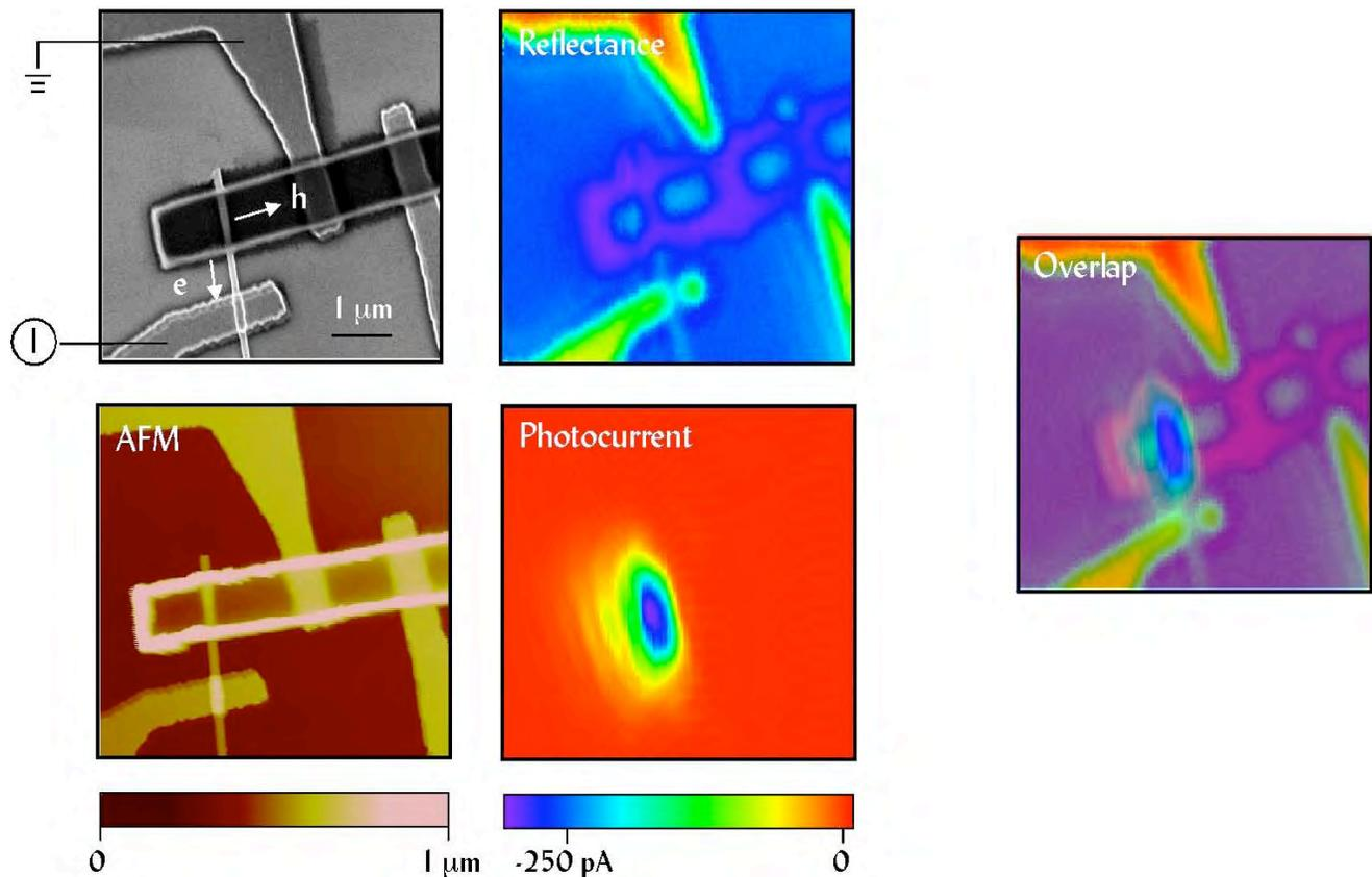
SEM (*upper left*), AFM (*lower left*), reflectance (*upper right*), and photocurrent (*lower right*) images of a single CdS-NW-P3HT heterojunction. These images clearly indicate that the photovoltaic action of CdS-NW-P3HT solar cell occurs entirely at the junction between the CdS NW and the P3HT polymer strip. The analysis of the photocurrent data as a function of laser wavelength provides information on the charge separation efficiency as a function of photon energy.
