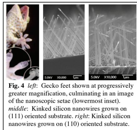
**Fig. 4** *left:* Gecko feet shown at progressively greater magnification, culminating in an image of the nanoscopic setae (lowermost inset). *middle:* Kinked silicon nanowires grown on (111) oriented substrate. *right:* Kinked silicon nanowires grown on (110) oriented substrate.
