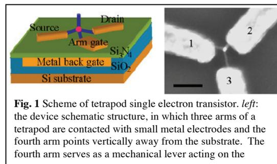
**Fig. 1** Scheme of tetrapod single electron transistor. *left*: the device schematic structure, in which three arms of a tetrapod are contacted with small metal electrodes and the fourth arm points vertically away from the substrate. The fourth arm serves as a mechanical lever acting on the
