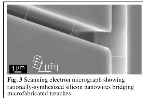
**Fig. 3** Scanning electron micrograph showing rationally-synthesized silicon nanowires bridging microfabricated trenches.
