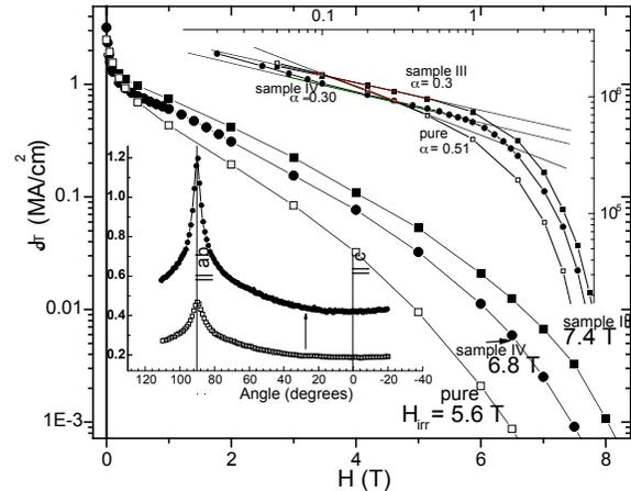
Fig. 2. Magnetic field dependence of transport critical current density  $J_{cT}$  at 77 K for  $B \parallel c$  of multilayered film, YBCO/(Y2O3/YBCO) x 9.<sup>2</sup>
