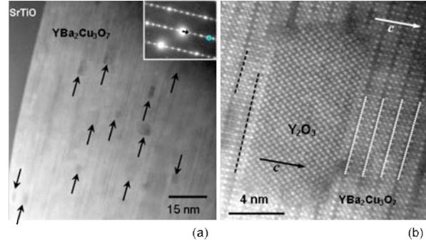
Fig. 1. STEM-images of (a) an YBCO film embedded with  $\text{Y}_2\text{O}_3$  nanoparticles (indicated by arrows) and (b) a coherent  $\text{Y}_2\text{O}_3$  nanoparticle in YBCO matrix.<sup>1,2</sup>
