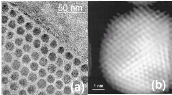
Fig. 3 (a) 3-D self-assembled Ni-nanoparticles in Al<sub>2</sub>O<sub>3</sub> thin film matrix. (b) STEM-image of a single Ni-nanoparticle in Al<sub>2</sub>O<sub>3</sub> thin film matrix.<sup>3</sup>
