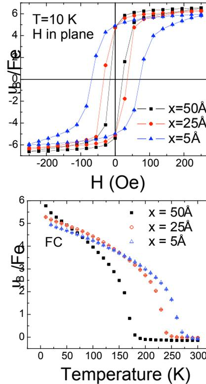
Fig. 4: Field (top) and temperature (bottom) dependence of normalized Fe moment Bohr magnetons for different  $x$ . The coercivity increases by a factor of 3.8 and the  $T_C$  by a factor of 1.6. The saturated moment for all  $x$  is enhanced by a factor of  $\sim 3$  over the value (2.1 Bohr magnetons) for pure iron.<sup>4</sup>
