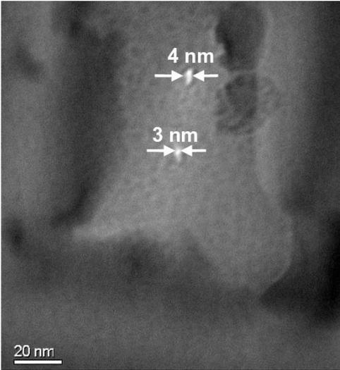
Figure 1: Transmission electron micrograph of a bi-nanopore device in a silicon chip (after oxidation). The light gray area is a thin layer of  $\text{SiO}_2$ . [4]
