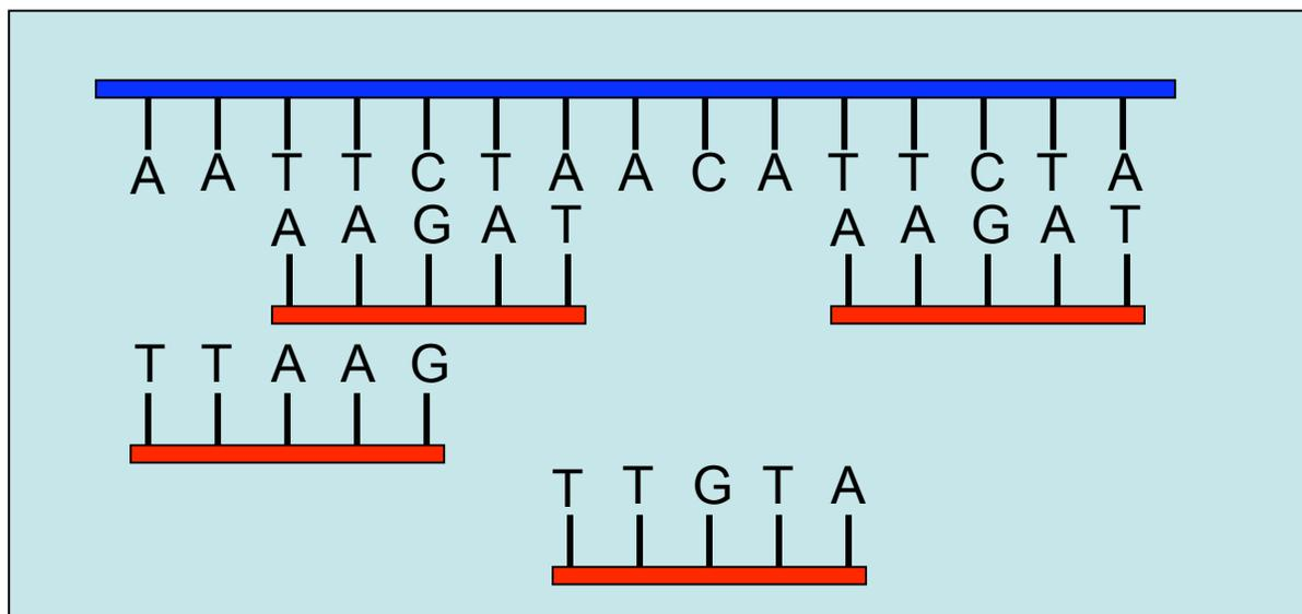
Figure 4: Hybridization-assisted nanopore sequencing of DNA. In this method, the position of each hybridizing DNA probe (in red), a short oligonucleotide, is determined from the ionic current trace using the standard patch-clamp electronics. The DNA sequence of the target DNA (in blue) can be constructed from the sequences of matching DNA probes and their positions.[3]
