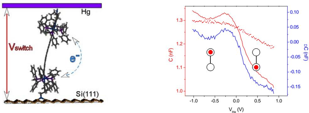
Figure. Capacitance measurements show single electron switching of QCA-active molecules. The measurement is the solid red line, the dotted red line is the control (unoxidized sample) and the blue line is the difference. The electron residing in the top or bottom dots represents a binary 1 or 0.
