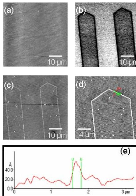
An AFM topography image (a) shows the surface of polarity patterned lithium niobate before a deposition. Using piezo-force microscopy, (b), the domain walls are the black lines between the lighter and darker domains. After the liquid phase process, AFM topography images (c, d) establish that silver nanowires have formed on the domain walls. The line profile (e) shows the wire to be about 250 nm wide.
