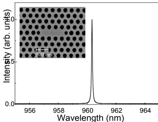
Fig. 1. Micro photoluminescence spectrum of the cavity mode under 780 nm cw excitation at a pump power of 3  $\mu$ W at 4.5 K. Inset: SEM of an L3-type photonic crystal microcavity with 260 nm lattice constant around the defect.
