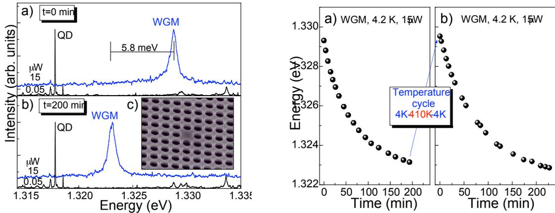
Fig 3. Left panel: slow S1 cavity mode drift of up to 6meV as a result of thin film deposition. Right panel: by increasing the temperature from 4K to 410K the film is removed and the cavity frequency is reset.
