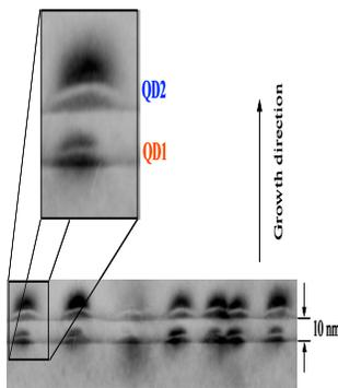
Fig 4. Strain-induced pairs of coupled QDs
