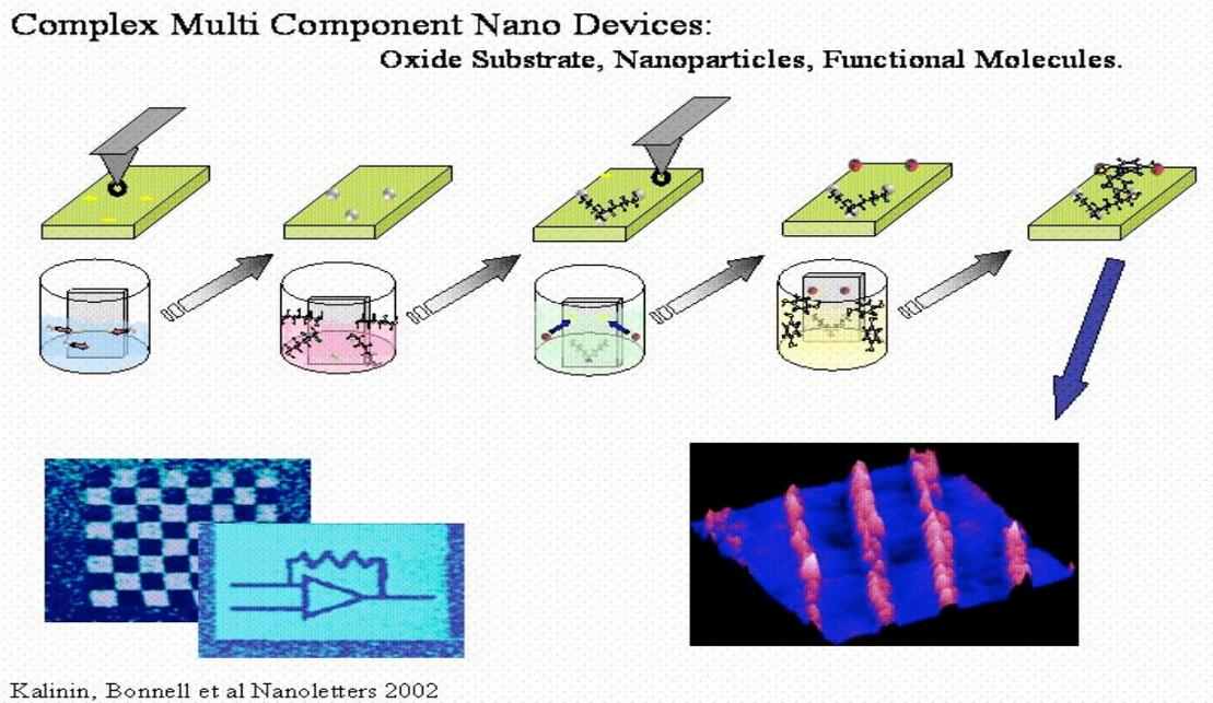
positive domain and participate in a reduction reaction. Oxidation can occur at a negative domain. In the case of photo reduction of metal, the reaction product is 3nm-30nm diameter
