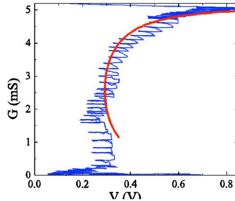
SEM images (left) of a nano gap electrode produced by controlled electro migration. The gap is not visible at this resolution. The conductance is used to monitor the process as the voltage is ramped.
