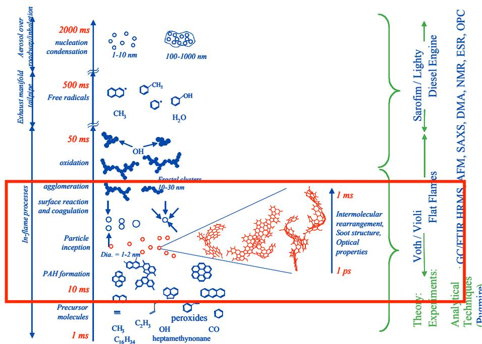
Fig. 1 (left) shows the “roadmap” for the project and illustrates the work which has been accomplished in Year 1 (boxed area). As seen in this figure, the work has focused on particle inception and agglomeration, optical properties, and experimental work on young soot.
