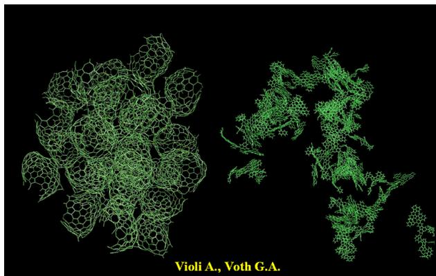
Fig. 2 (left) shows an example of the simulation, for two different agglomeration geometries. Round particles (left) tend to cluster, while “flaky” particles behave differently and tend to subcluster. These simulations, combined with experimental results, will begin to help validate the agglomeration kinetics of soot particles.
