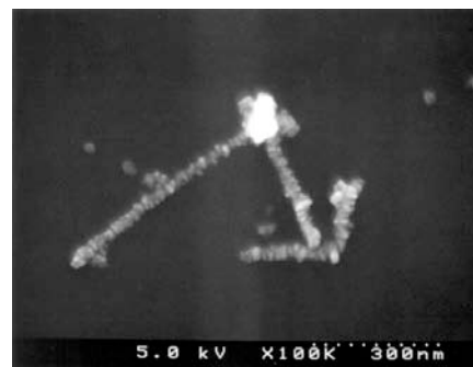
Fig. 4: Microtubules metallized with Cu imaged using scanning electron microscopy (SEM). The presence of copper particles on the microtubule surface was confirmed using energy-dispersive spectroscopy (EDS). The thickness of the Cu coating ranges from 5 to 45nm.
