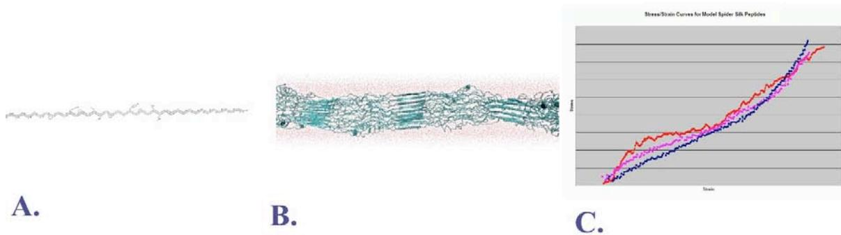
Figure 4. A. is the model of a single spider silk protein molecule. B. is an assembly of molecules and C. shows the stress-strain curve for the single molecule (blue) and assembly (pink) from computer simulation and fiber (orange) from mechanical testing.
