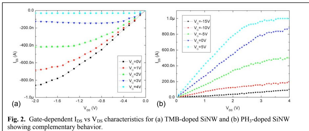
**Fig. 2.** Gate-dependent  $I_{DS}$  vs  $V_{DS}$  characteristics for (a) TMB-doped SiNW and (b)  $\text{PH}_3$ -doped SiNW showing complementary behavior.
