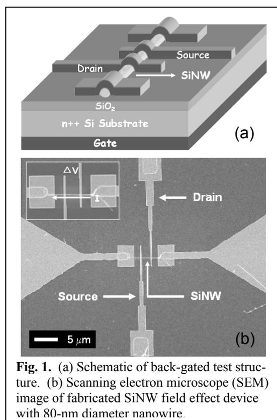
**Fig. 1.** (a) Schematic of back-gated test structure. (b) Scanning electron microscope (SEM) image of fabricated SiNW field effect device with 80-nm diameter nanowire.
