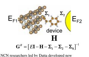
techniques to simulate electronics conduction through molecules on silicon. This group predicted that such devices would display novel electronic characteristics (negative differential conductance) that were recently confirmed experimentally.
