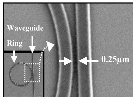
**Fig. 3.** Scanning electron micrograph that shows the top-view of a ring resonator coupled to a waveguide. Inset shows the entire ring structure. A pump pulse incident on the ring structure controls the transmission properties of a signal pulse sent through the waveguide.
