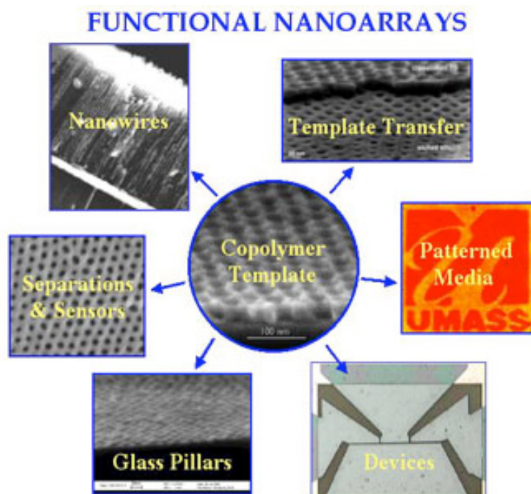
Figure 1. Several application areas enabled by the diblock copolymer nanoporous template fabrication method.
