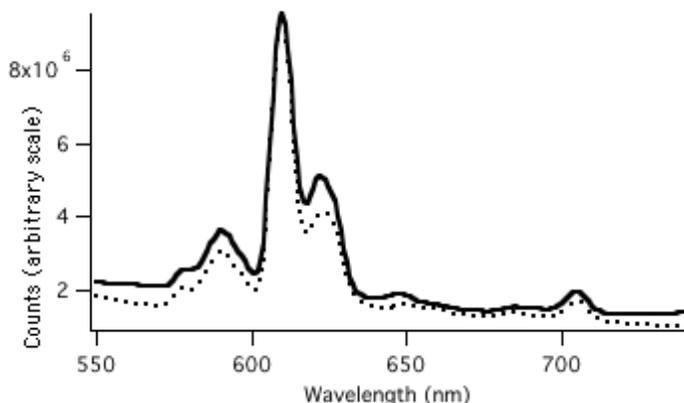
Figure 2 Emission spectra of untreated (full line) and functionalized (dashed line) Eu<sub>2</sub>O<sub>3</sub> nanoparticles
