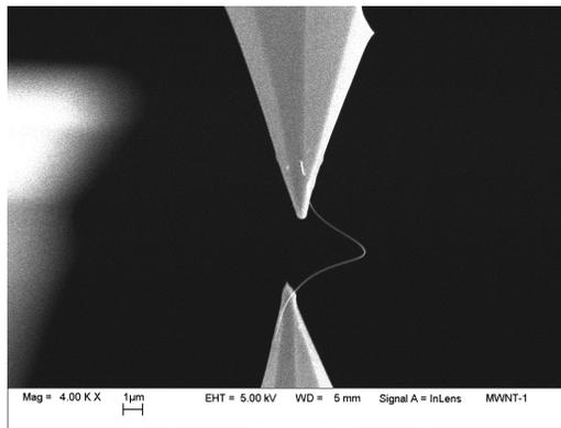
up, mount, and tensile load carbon nanotubes such as the individual multiwalled carbon nanotube shown attached between AFM cantilever tips (right image). We have reported on the breaking mechanism and tensile strength of MWCNTs [1], the tensile strength of single wall carbon nanotube ropes [2], and “shell sliding,” in which the outer shell of a MWCNT is displaced relative to the inner shell adjacent to it [3, demonstration of a nanobearing].
