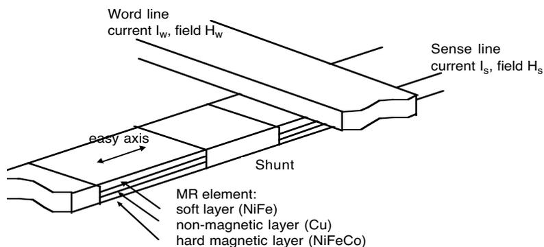
Schematic of MRAM structure, which consists of an array of parallel sense lines and parallel word lines. The MR elements are connected in series. Magnetic fields generated by currents passed simultaneously through a sense line and a word line write the element at the intersection of the two lines. To read, resistance changes in the sense line caused by a smaller wordline current are measured.
